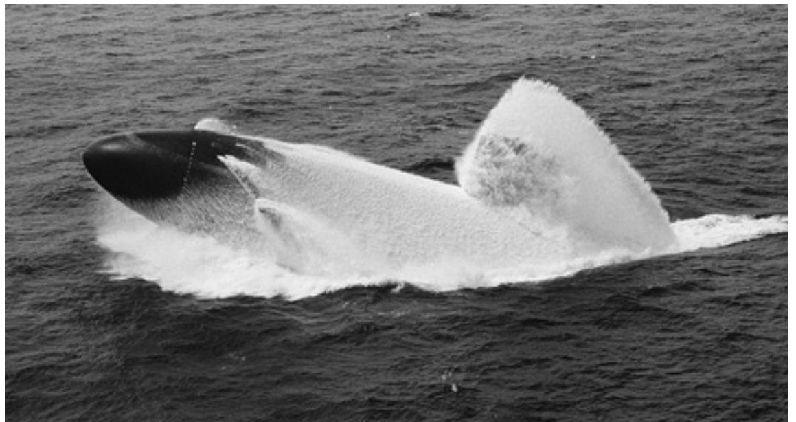
A nuclear submarine broaching following a test of its emergency blow system. High pressure air is used to force water out of the sub's ballast tanks, resulting in the sub becoming so buoyant that it is almost thrown out of the water.
